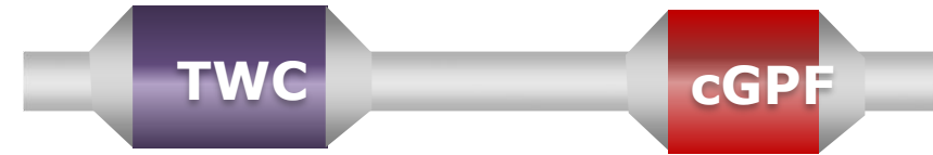
Three Way Catalyst (TWC) plus coated Gasoline Particulate Filter (cGPF)
