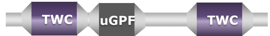
Three Way Catalyst (TWC) and uncoated Gasoline Particulate Filter (uGPF) plus downstream TWC
