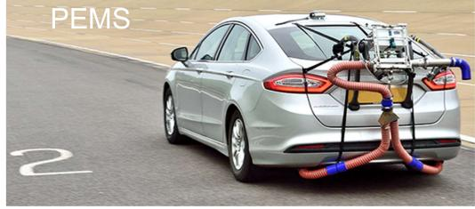
• Cambustion emissions analyzers have a response time of a few *milliseconds (...a thousand times faster)*
